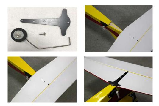
3. Punching the hole which threading the tail wheel wire to plug in rudder; Threading the tail wheel wire from the bottom to the top; Stick the rudder into the tail wheel wire, and insert the rudder hinge into fuselage hinge slot; Use 502 gluing and fixing it.
