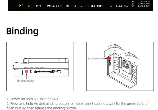
3. Press the VRX frequency-binding button/M button for more than 3 seconds, wait for the
