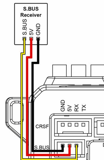
The S.BUS port provides output from a stabilized 5 V rail, which is a common working voltage for S.BUS type receivers. Verify that your receiver supports 5 V before powering it up through OFS3 for the first time. The connector type used is Picoblade 3-pin, but is also compatible with JST MX 1.25mm connectors.
