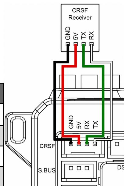
The adjacent diagram illustrates the required connection between the CRSF receiver and flight controller. Note that it is possible to fly with the receiver's TX pin connected only, but no telemetry will be returned.
