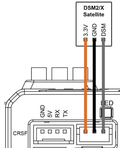
The DSM port provides output from a stabilized 3.3 V rail, which is a common working voltage for DSM receivers. Verify that your receiver supports 3.3 V before powering it up through OFS3 for the first time. The connector type is JST-ZH 3-pin.
